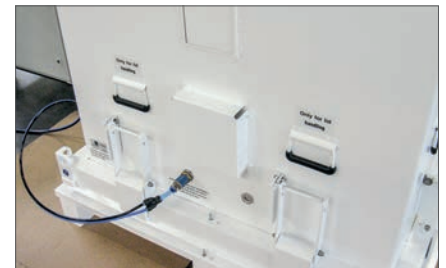
Water-vapour-proof container being leak-tested with overpressure
